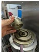
The HiDiff-X integrates a quick tool changer interface allowing the mechanical re-centering and electrical connection of different tools on top of the Centering stages. No tools are required to switch from Fixed sample holder to Kappa/Phi head or plate holder.
